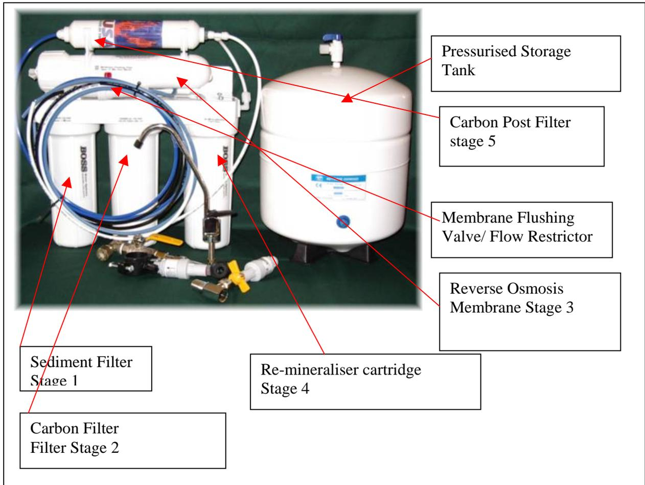
**Stage 1** Sediment pre-filter, this filter is a 1 micron polyspun sediment filter cartridge for mechanical removal of Grit, dust, Rust, mud, algae ect. This cartridge is normally replaced every 12 months but if dirty mains water is encountered more frequent change may be required.
